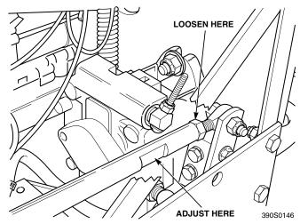
Figure 6-4. LH Steering Control Rod Adjustment
